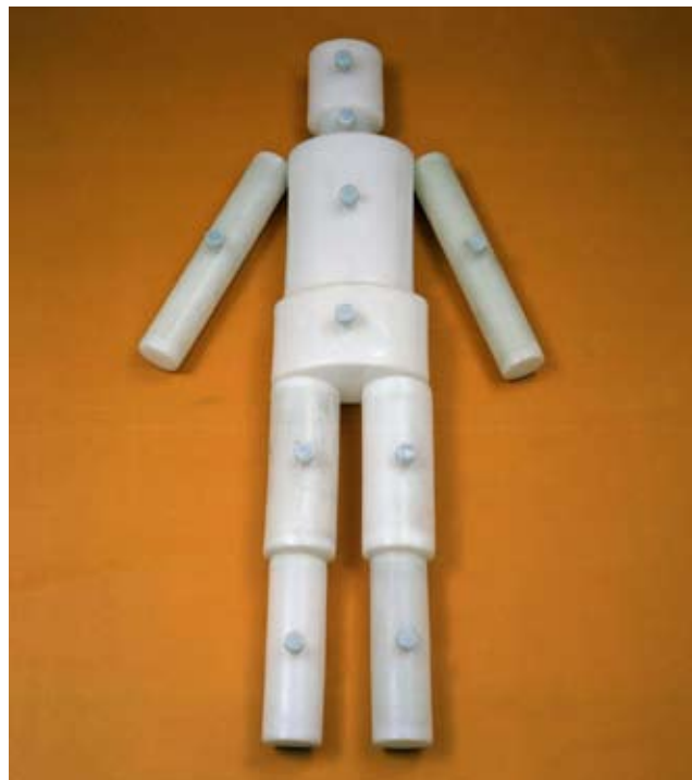
Figure 3: The bottle manikin absorption (BOMAB) phantom simulates Reference Man in size and internal body density. It is used to “calibrate systems used to detect and quantify the amount of radioactive materials in workers.” BOMAB is loaned to DOE sites by the Pacific Northwest National Laboratory. Phantoms for a Reference Female and four-year old child are also available. (Sources: http://picturethis.pnl.gov/pictureet.nsf/by+id/AMER-5XBN9N , http://www.pnl.gov/phantom , and http://www.pnl.gov/phantom/bomab )
